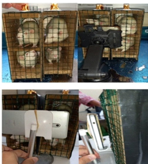
Figure 1. The mobile phone devices are placed within a 3 cm distance from the cage which the electromagnetic exposure effect observe.
